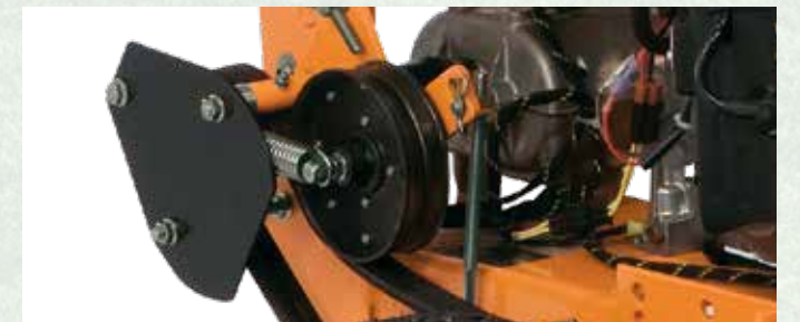
Twin power belts provide double friction to pulley surfaces and reduce slipping in wet conditions.
