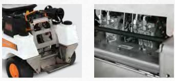
Removable cushion and open lower area allow quick and easy service access to the hydro drive pumps, hydro oil reservoir and other mechanicals.
