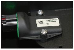
Onboard Bluetooth capabilities offer remote troubleshooting through the Smartec Connect™ and Smartec MyMow® apps.
