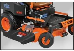
Fully-fabricated and welded 52" Hero™ cutter deck provides an envy-inducing quality-of-cut.
