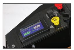
Full-featured display screen shows battery charge level, hours of run time and provides system diagnostics.
