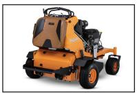
Spacious operator platform with suspension and padded, bolstered cushion for a smooth, comfortable ride.
