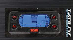
The Tiger Eye™ Advanced Monitoring System keeps a constant, real-time "eye" on important system functions of your AerStorm. The system features blue backlighting for low-light conditions, yet has high contrast visibility in full sunlight. IP 67 rated water and dust proof with a scratch-resistant lens for worry-free performance in any conditions.
