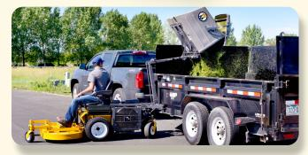
The Walker Hi-Dump® raises 67 inches and dumps collected grass and debris into a truck or trailer with a 20-second cycle time.
